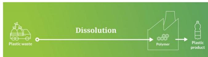
**'Dissolution' / 'Solvent based purification' / 'Solvent based extraction'** - Sorted plastic waste is dissolved to extract the polymers and make new recycled plastic from them.
