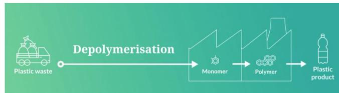
**'Depolymerisation' / 'Chemolysis' / 'Solvolysis'** - Sorted plastic waste is broken down into monomers to feed them back into the plastic production.
