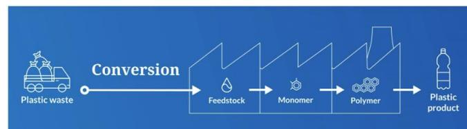
**'Conversion' / 'Pyrolysis' / 'Gasification'**- 'Mixed' plastic waste is broken down into oil- or gas-like feedstock used to produce chemicals including plastics
